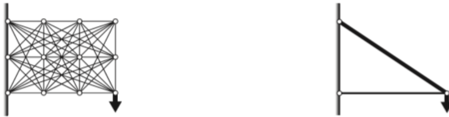
Figure 5.12: [27] The left side is a ground structure and the right hand side is an optimal solution obtained from the ground structure method.
